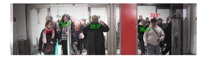
These thermal cameras have a very advanced and effective algorithm for high precision mesuring. It has an Al based on facial recognition. This allow to filter all types of false alarm that could be generated by any other warm objects (cigarettes, coffees, lights, etc.).
